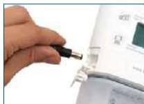
Plug the Invia Motion power supply into a wall outlet and open the small protective cover of the pump for the Direct Current (DC) socket and attach the power supply. Moving bars on the battery display will indicate charging is occurring. [ ].
