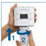
3. Make sure the canister is aligned with the label to the front.
